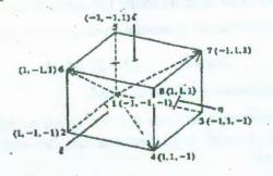
16. a) Determine the strains developed in elastic body when it is strained. The following figures [5] show the undeformed and deformed shape of the body.
